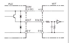
Note: 1. Use the M7F positive logic input model if the PLC Output Unit has PNP output.
