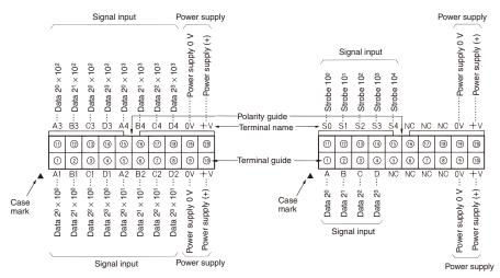
**Note:** Circled numbers are for the user's convenience. When preparing a socket, pay attention when wiring the terminals to the direction of the polarity guide.
